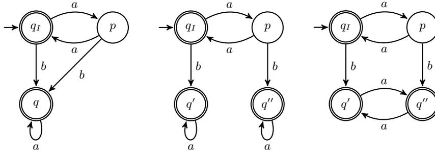
**Fig. 1.** A minimum DFA accepting the language  $L = (aa)^* + a^*ba^*$ , with two minimal nonisomorphic REV-DFAs. In the DFA on the left the reversible part consists of the states  $q_I$  and  $p$ , while the irreversible one of the state  $q$ . The REV-DFA in the center is obtained by the algorithm in [3].
